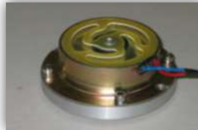
Low tech /cost „body shaker“ (acoustic absorber)
