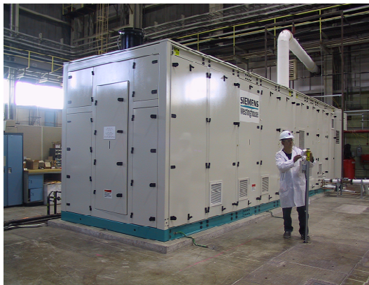
CHP250 SOFC Power System for Ontario Power Generation (2292 cells, 225 kWe @ efficiency > 45%, 250 kWe max)
