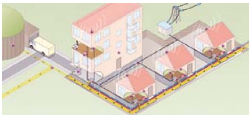
The FC-DISTRICT concept: Intelligent Heat Network with SOFC micro-CHP units
